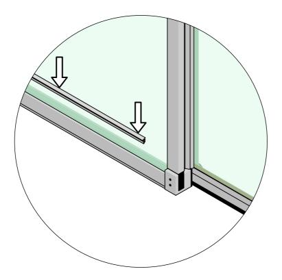
Adjust and tighten both door stoppers.
