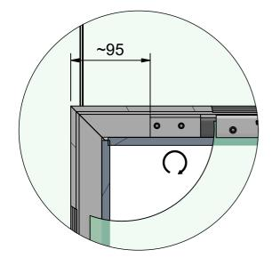
Check that the automatic threshold closes tightly when door is shut.
