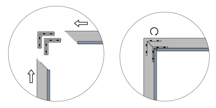
and attach it to main frame. Tight the 8 x M5 screws using max torque 2 Nm.
