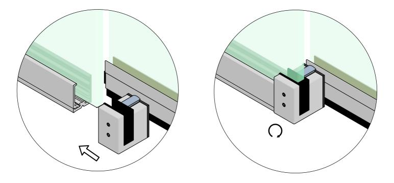
Attach outer door guide leaving some space to the threshold.
