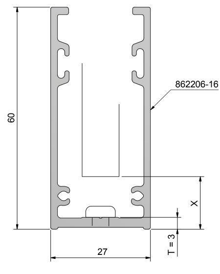
X = Deduction for glass (floor) = T + glazing blocks height X = Deduction for glass (wall or ceiling) = T + screw height + clearance
